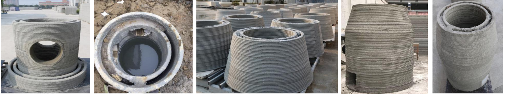
WINSUN's First Generation 3D printed Double-Layers Sewage Wells
